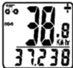
**ODOMETER (ODO)**— Total distance traveled is indicated by “ODO” and displayed on the bottom line. To reset ODO, press the LEFT button for 2 seconds or remove and replace the battery. Adjust each flashing digit by pressing the RIGHT button and then press LEFT to confirm. Now press the RIGHT button to advance to the DST mode.
