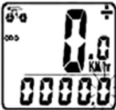
**TRIP TIMER (TM)** – Trip Timer is indicated by TM and is displayed on the bottom line. The Trip Timer is activated automatically with computer input (comes on automatically when you begin riding, turns off when you stop). It records only the time actually spent riding. To reset TM to zero, return to DST (Trip Meter) mode and reset to zero per the instructions above. Return to TM mode and press the RIGHT button to advance to the Temperature mode.
