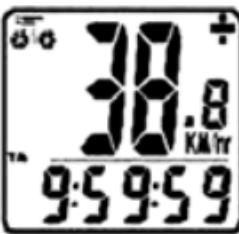
**TEMPERATURE (TEMP)** – Your computer has a thermometer to measure outdoor temperature. To select between Celsius (C) and Fahrenheit (F) readout, press and hold the LEFT button for 2 seconds. Press the RIGHT button to select between C and F and press the LEFT button to confirm. Now press the RIGHT button to advance to the (CAL) mode.
