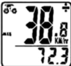
**MAXIMUM SPEED (MXS)**— Maximum speed is indicated by MXS and is displayed on the bottom line. Maximum speed is stored in memory and updates only when a higher speed is reached. To reset MXS, press and hold the LEFT button for 2 seconds. Now press the RIGHT button to advance to the Average Speed (AVS) mode.
