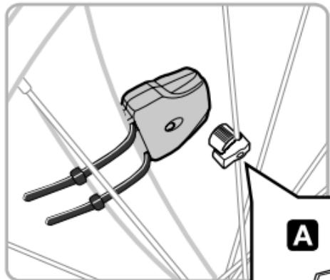
Secure the magnet to a spoke on the right side of the front wheel. Clamp will work with both **(A)** thick and **(B)** thin spokes. Screw to attach. *Make sure magnet faces toward the outside of the wheel.*
