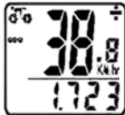
**SPEEDOMETER** – Instantaneous Speed is indicated on the top line. The range of measurement is from 0 to 99 KM/hr (0 to 99 M/hr) and accuracy is  $\pm 0.5$  KM/hr (M/hr).
