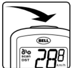
**EL BACKLIGHT** – illuminates the computer screen for easier viewing in dark or low light settings. To turn it on tap the center button on top of the cabinet.
