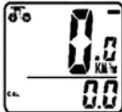
**CALORIES BURNED (CAL)**— This function estimates the number of calories burned while riding, based on the age and weight inputted by the user. To reset CAL, press and hold the LEFT button for 2 seconds. Now press the RIGHT button to advance to the (FAT) mode.
