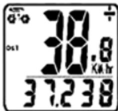
**TRIP METER (DST)**— Trip distance is indicated by DST and is displayed on the bottom line. The Trip Meter is activated automatically with speedometer input (comes on automatically when you begin riding, turns off when you stop). To reset DST to zero, press and hold the LEFT button for 2 seconds. Note that TM (Trip Time) & AVS (Average Speed) will also be reset at that time. Now press the RIGHT button to advance to the MXS mode.
