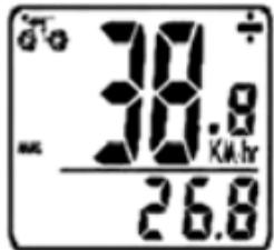
**SPEEDOMETER COMPARATOR** – A "+" or "-" sign appears to the right of the speed. "+" indicates you are travelling faster than your average speed (AVS). A "-" indicates you are riding slower than your average speed.
