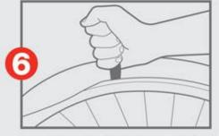
The last little bit of tire will be hard to get into the rim, use your tire lever to pry over the rim's edge.
