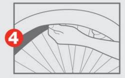
Insert the valve of the new tube through the valve hole then work around the tube pushing it into the tire as you go.
