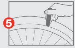
Once the new tube is inside the tire, reset the tire back inside the rim using your hands and tire levers.
