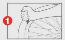
Loosen your brakes and remove the wheel of the punctured tire from the bike and lay it flat on the ground. Use the thin end of your first tire lever to pry the tire onto the outside of the wheel's rim.
