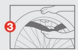
Pull out the old tube by reaching between the rim and the tire and then discard the old tube. Using your hand, carefully feel around the inside of your tire to ensure there is nothing sharp which will cause another puncture. BE CAREFUL!
