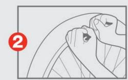
Insert your second tire lever in the same manner a few spokes to the right, then move the two tire levers apart from each other along the rim of the wheel bringing the entire side of the tire outside of the wheel.
