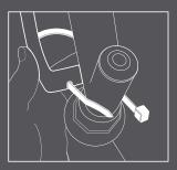
THREAD ZIP TIE THROUGH HOLES OF BRACKET ARM AND AROUND HANDLEBAR STEM TO SECURE.
