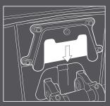
INSTALL BRACKET BY SLIDING BASKET GROOVE DOWN ONTO TOP OF BRACKET – RED BUTTON WILL POP OUT AND MAKE A "CLICK" SOUND WHEN PROPERLY INSTALLED.
