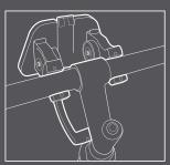
TO ADJUST BASKET ANGLE, MOVE SWING ARM TO DESIRED LOCATION AND RETIGHTEN SILVER BOLTS WITH 4 mm ALLEN WRENCH.
