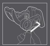
USE 4 mm ALLEN WRENCH TO LOOSEN SILVER BOLTS AT SIDES OF BRACKET SO THE SWING ARM MOVES.
