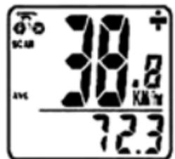
**SCAN**— The Scan mode conveniently rotates DST, MXS, AVS, and TM readings on the computer screen without the need to press any buttons. Now press the RIGHT button to advance to the Clock mode.
