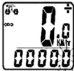
**AUTO STOP/START** – To preserve batteries, the cycle computer will automatically switch off if the unit is left unused for over 5 to 6 minutes. Display will reappear with a press on any button.
