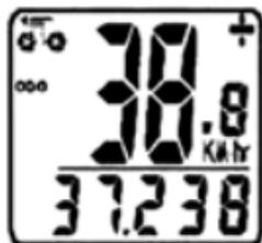
**ODOMETER (ODO)** – Total distance traveled is indicated by “ODO” and displayed on the bottom line. To reset ODO, press the LEFT button for 2 seconds or remove and replace the battery. Adjust each flashing digit by pressing the RIGHT button and then press LEFT to confirm. Now press the RIGHT button to advance to the DST mode.
