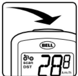
**EL BACKLIGHT**— illuminates the computer screen for easier viewing in dark or low light settings. To turn it on tap the center button on top of the cabinet.
